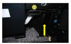
3. Remove dirty filter from housing carefully as accumulated debris may come loose. Clean housing of possible objects like leaves and insert new filter in the right air direction as indicated on the filter.
