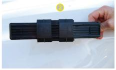
The filter housing sits underneath the glovebox on the right hand side of the footwell. Once housing has been indentified, slide the plastic braces towards the centre of the lid to release it as indicated in the picture above.
