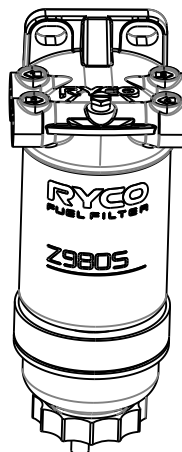
SECTION 2 FUEL WATER SEPARATOR
