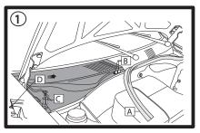
Remove the rubber seal (A), pull out the split pin (C), push spring locks (B) towards wind-screen, lift the cover to clear spring locks and slide the plug (D) and cover out to remove.
