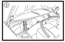
Remove used filter & replace with new Ryco RCA144P. Squash element as shown in 4 to remove & fit into housing.
