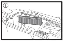
Remove used filter noting flow direction, replace with new Ryco RCA144P.
