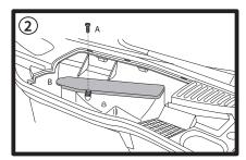
Remove the screw (A), hold the cover at the rounded end (B) pull upwards and remove filter cover.
