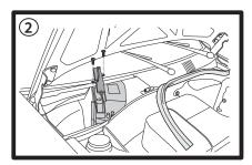
Remove the two hex headed screws and remove the filter housing lid.
