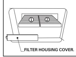
REMOVE FILTER HOUSING COVER, REMOVE AND REPLACE USED FILTERS (NOTE FLOW DIRECTION).
