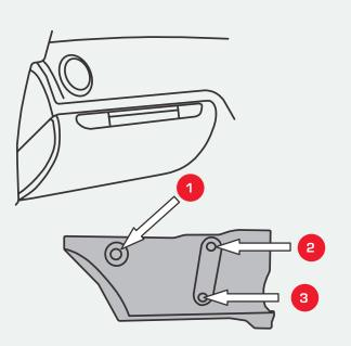
STEP 1 Filter is located under glovebox, remove panel by unlocking in 3 places as shown.
