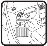
3 Pull dirty filter down to remove, push new Ryco filter up in to housing.
