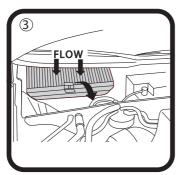
Undo clip, remove used filter, noting flow direction
