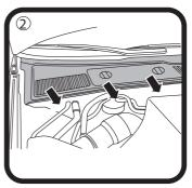
Pull cover towards front to expose filter housing.
