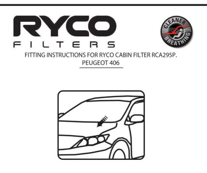
1. The cabin air filter is located in the engine bay below the windscreen inside the engine cowl.
