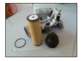
The sealing rod must be pushed all the way into the drain hole
