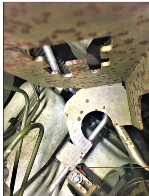
FIG. 18 RYCO AIR BOX BOLT & WASHERS FITTED
