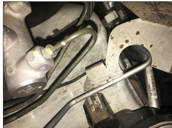
FIG. 17 FB9813CC FITMENT LOCATION, BEHIND AIR BOX VIEW
