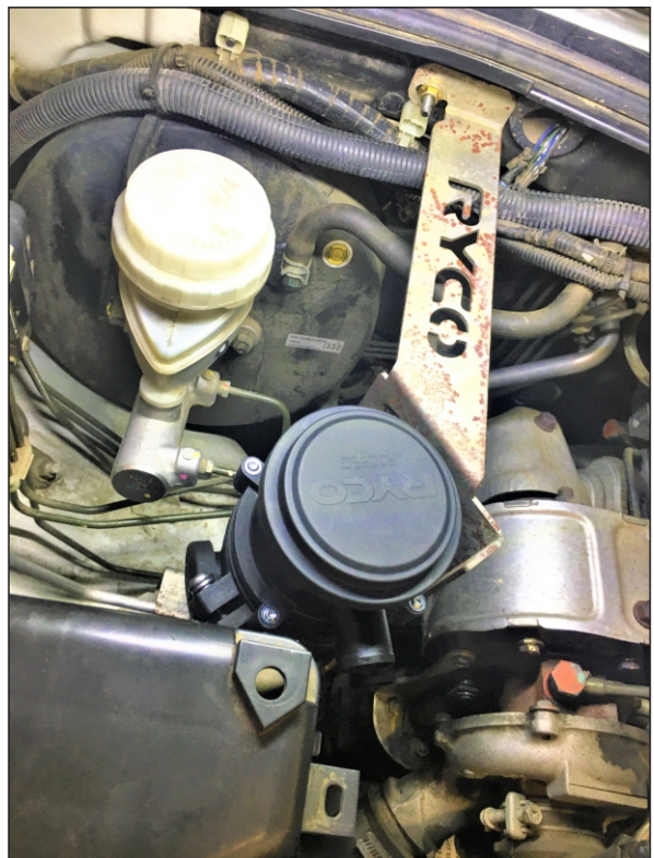
FIG. 20 CATCHCAN FITTED TO CATCHCAN BRACKET
