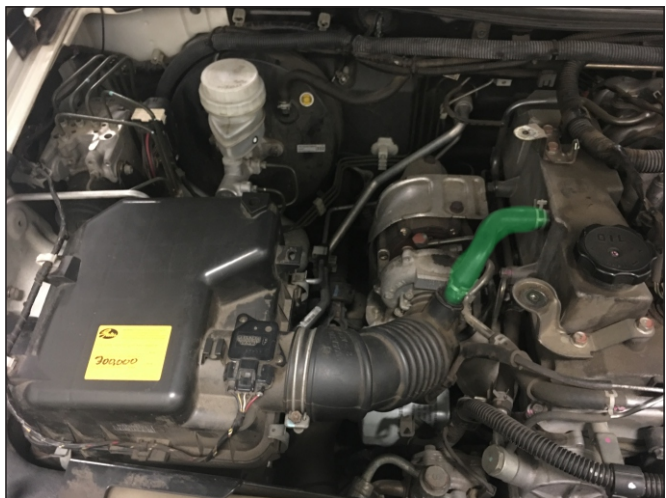
FIG.12 OEM PCV HOSE REMOVAL
