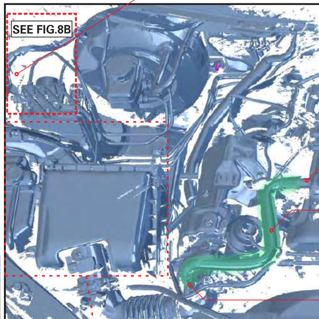
FIG. 8A OEM PCV HOSE REMOVAL
