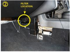
The filter is located on the rear end area of the centre console behind the side carpet panel. See Fig 3 for details.
