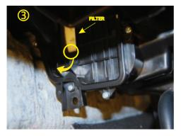
Release the housing cover by depressing the Hold the middle of new filter (A) and squeeze locking tab at the lower end and sliding it downwards. Carefully tuck out the bottom corner of old filter and squeeze & pull it out.
