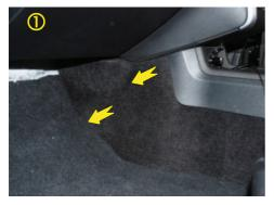
Remove side carpet panel in the passenger side footwell by lifting from front and then pulling the entire panel backwards.
