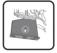
3 Pull dirty filter out to remove, push new Ryco filter into housing.
