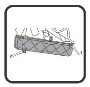
② Unlock in 2 places as shown, remove filter cover.
