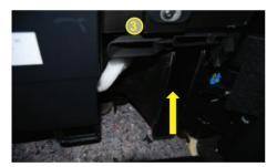
Remove dirty filter from housing slowly as dirt may be released onto the carpet. Clean the housing of possible objects like leaves and insert new filter in the right direction. Check flow direction indicated on filter.
