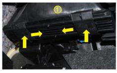
The filter housing sits underneath the glove box on the right hand side of footwell. Once housing has been identified slide plastic braces towards the centre of the lid to release it as indicated in the picture above.
