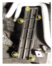
With a Phillips screw driver remove the four screws holding the cabin air filter housing lid and remove lid.
