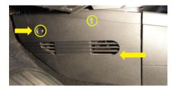
The cabin air Filter is located on the passanger footwell behind the centre console lower trim. Remove clip and slide forward to remove.
