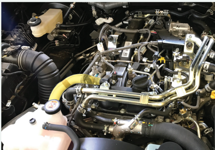
FIGURE 3 FACTORY PCV HOSE POSITION AT ENGINE BAY
