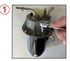
1. Undo the 6 T20 Torx bolts from the fuel filter housing.
