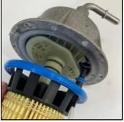
3. Push the new filter against the housing. Make sure the breather pipe lines up with the breather hole.
