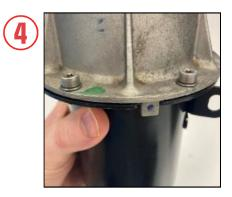
4. Put the filter back in place and tighten the 6 T20 Torx bolts.
