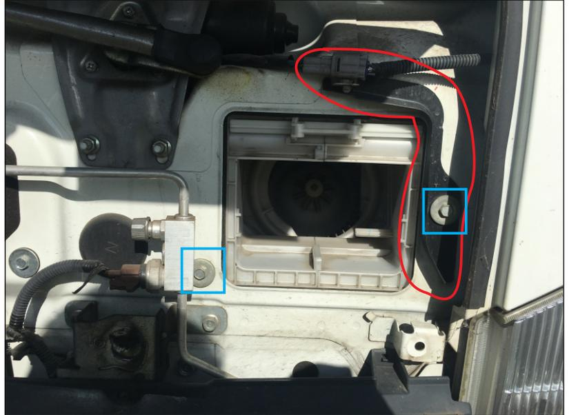
**FIG. 14 BOLT AND BRACKET REMOVAL**
