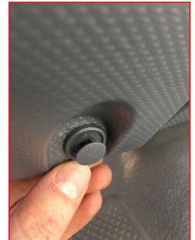
FIG. 6 PASSENGER DASHBOARD CLIP REMOVAL
