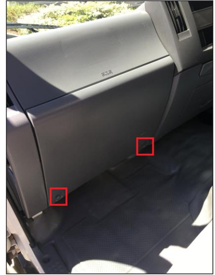
FIG. 5 PASSENGER DASHBOARD REMOVAL
