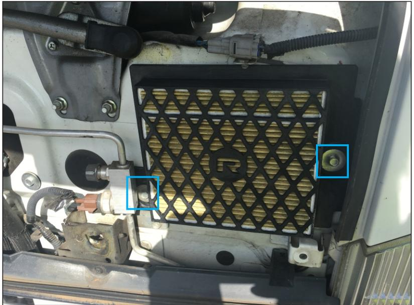
**FIG. 15 BOLT AND BRACKET REMOVAL**
