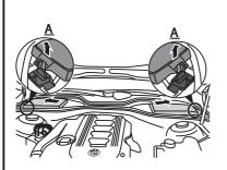
OPEN BONNET, LOCATE HOUSING, UNCLIP LID AND LIFT UP AT ARROW "A" THEN REMOVE, LIFT AND PULL USED FILTER TOWARDS SIDE OF VEHICLE TO REMOVE.
