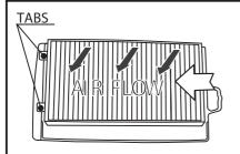
CHECK AIR FLOW DIRECTION, THEN PUSH FILTER INTO PLACE ENSURING BOTH TABS ARE LOCATED IN END OF HOUSING, REPLACE LID, REPEAT FOR OTHER SIDE.
