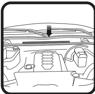
1. The cabin air filter is located in the engine bay towards the passenger side.
