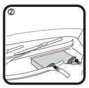
Fit new filter and frame into housing, push clips to lock, close cover and replace weather strip.
