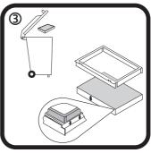
Dispose of used filter, fit new RCA118C to frame, ends of frame fit into last pleat at ends of filter.
