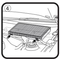
Fit new filter and frame into housing, push clips to lock, replace cover, screws and weather strip.
