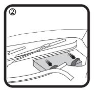
Undo 2 clips by pulling to front of vehicle, remove filter and frame.
