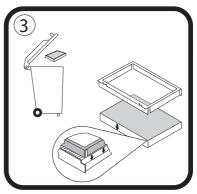
Dispose of used filter, fit new RCA118C to frame, noting flow direction.
