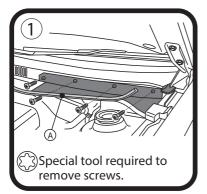
Remove weather strip (A) undo 4 screws and remove cover by pulling forwards.
