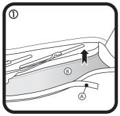
Remove weather strip (A) and fold cover back (B)
