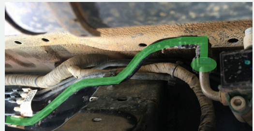
FIGURE 2B OEM INLET FUEL LINE REMOVAL (OEM FILTER HOUSING VIEW)
