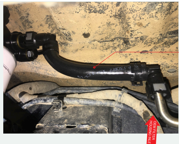
FIGURE 4C HF9805B HOSE INSTALLATION
