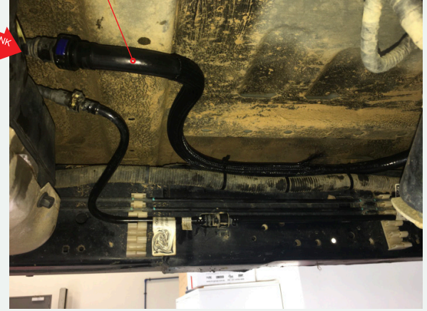
FIGURE 4A HF9805A HOSE INSTALLATION (FUEL TANK SIDE)
