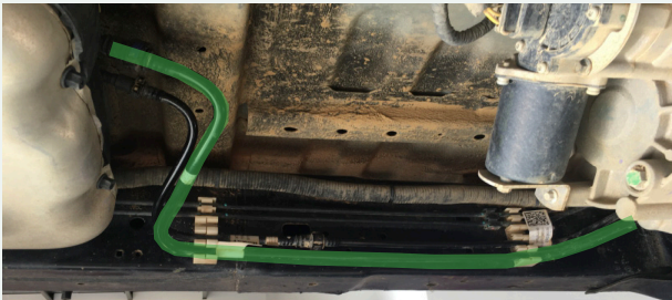
FIGURE 2A OEM INLET FUEL LINE REMOVAL (TANK VIEW)
