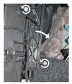
Remove housing cover bolts and housing cover.
