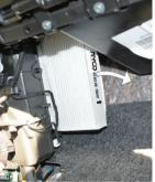
4. Insert the new filter into the housing.
