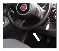
1.The cabin air filter housing is located at the front of . the centre console adjacent to the right footwell.
