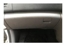
1. The cabin air filter housing is located behind the glove box. To gain access, the glove box must be lowered from the upper stops.
