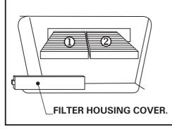
REMOVE FILTER HOUSING COVER, REMOVE AND REPLACE USED FILTERS. ENSURE ARROW ON SIDE OF FILTER IS POINTING UP.
