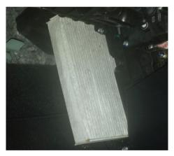
Pull the old filter out and replace with Ryco cabin air filter. Making sure it is in the right direction. See the side of the filter for direction indication. Refit all components in reverse order.
