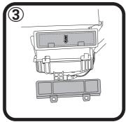
Unclip filter cover and remove, pull used filter out of housing and replace with new Ryco filter.
