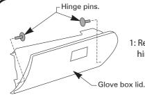
1: Remove glove box lid by levering hinge pins out as shown.
