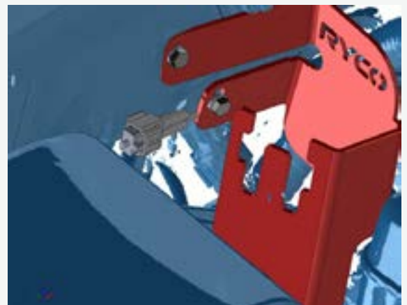
FIGURE 2C CATCH CAN BRACKET SLOT B & C INSTALLED
