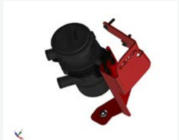
FIGURE 3B CATCH CAN INSTALLED
