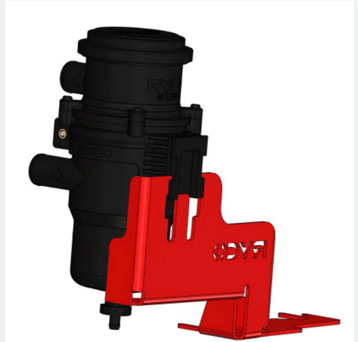
FIGURE 3A CATCH CAN BRACKET INSTALLATION
