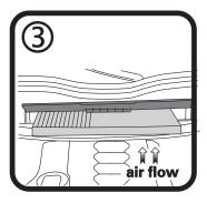
Pull filter towards front of vehicle and remove, Fit new Ryco RCA135M. Ensure arrow points up. Close and lock housing door.
