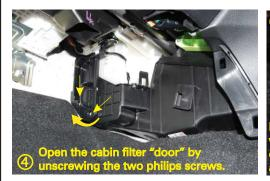
Ryco Group Pty Ltd 29 Taras Ave Altona North Victoria 3025 Australia. www.rycofilters.com.au Remove the old filters. Insert the new filter with foam on its top and push up into the compartment. Slide and snap the other filter and refit all parts in reverse direction.
