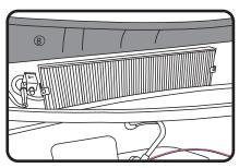
2: Lift cover panel B and fold back to expose the filter
