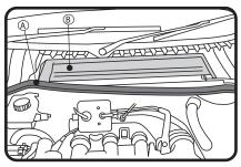
1: Lift weather strip (part A) from ridge for length of cover panel. (Part B).
