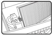
3: Undo clip at both ends of housing and remove used filter.
