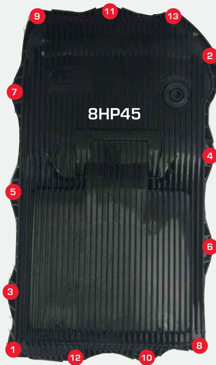
FIGURE 1 TIGHTENING TORQUE FOR SCREWS ON A PLASTIC OIL PAN = 10 Nm \pm 1.0 Nm.
