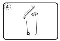
4:Refit components in reverse order, Dispose of used filter correctly.
