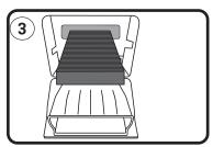
3:Remove used filter and replace with a new Ryco filter. Note direction of flow arrow printed on filter.
