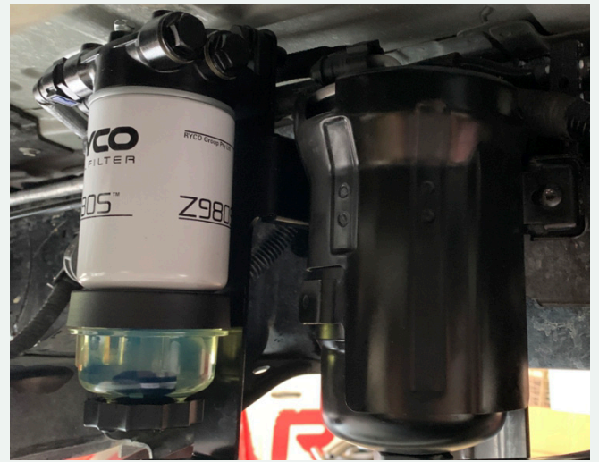
FIGURE 8C FUEL HOSE INSTALLATION - FUEL WATER SEPARATOR END SIDE
