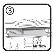
Pull filter towards front of vehicle and remove, Fit new Ryco RCA135C. close and lock housing door.
