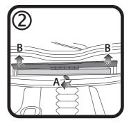
Unlock at "A" then swing door open by holding at "B" and lifting.
