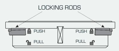
OE FILTER LOCKING / UNLOCKING RYCO FILTER LOCKING / UNLOCKING
