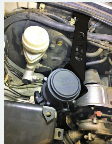
FIGURE 10 CATCH CAN FITTED TO CATCH CAN BRACKET
