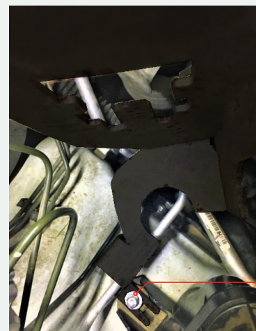
FIGURE 8 RYCO AIR BOX BOLT AND WASHERS FITTED
