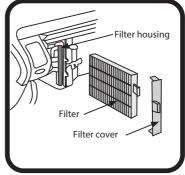
3:Remove the filter cover from housing, Remove used filter and replace with new Ryco cabin air filter. Refit filter cover making sure filter is seated correctly, refit the glove box frame.
