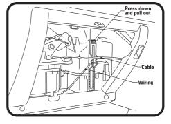
2: Remove cable and wiring from filter cover plate, push down and pull out to remove cover plate.
