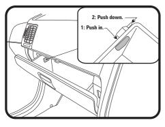
Open glove box and remove retaining pins on either side of glove box, then fully open glove box.
