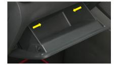
2. Release the glove box upper clips by pushing the upper glovebox inboard as shown in the diagram.
