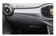
1. The cabin air filter housing is located behind the glovebox. To gain access, the glovebox must be opened and lowered.
