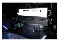
4.Insert the new filter into the housing. The UP arrow indicates the position direction. Refit all components in reverse order.
