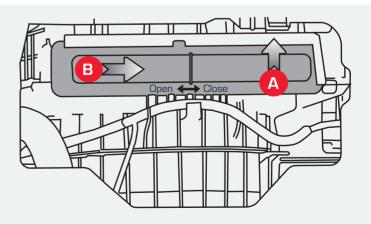
**STEP 5** Install new filter cover in position,insert into the upper slot (direction A) and secure by moving the cover to the right (direction B) if fitting for first time, or use old cover. Refit all previously removed components.
