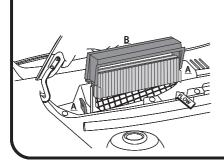
Release 2 clips (A), lift cover (B) to remove, remove used filter from housing and replace with Ryco RCA134P, note direction of air flow Replace all previously removed components
