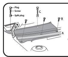
Lift rubber seal (A) from ridge then remove 3 screws (B), remove 2 caps, 2 screws and 2 split plugs (C), remove cover from vehicle.
