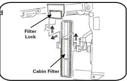
3. Push new RYCO filter (2 pcs unit) into filter housing (Ensure the air flow arrows are pointing to left hand side of the vehicle). Refit filter lock, stay bracket and glove box.
