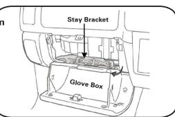
2. Remove filter lock as shown and pull the old cabin filter outwards from the housing.
