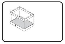
3: Fit new Ryco RCA103P into frame noting that ends of frame fit into pleat space both ends
