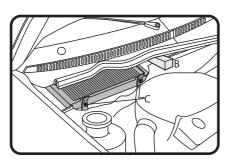
2: Use approx 50mm high support (B) to keep weather strip clear of filter push clips (C) towards engine, lift front of filter assembly and pull out of housing.
