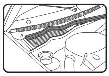
1: Lift weather strip (part A) from ridge to at least centre of vehicle.
