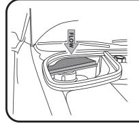
Pull used filter out from housing then fit new RYCO RCA157P by pushing into housing, Note air flow direction and positioning of filter.
