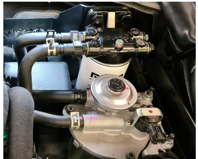
10. Start the engine and check the Z980SK16 fuel filter, fittings and hoses for any leaks.
