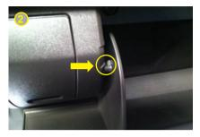
Open the glove box. With both hands positioned in both upper corners of the compartment just above the arrow on the picture, apply some force in the arrow direction to unhinge the compartment retaning lugs. Once that is done it will drop completely.
