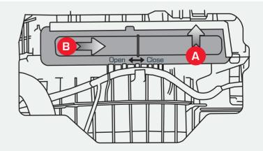
**STEP 5** Install new filter cover in position,insert into the upper slot (direction A) and secure by moving the cover to the right (direction B) if fitting for first time, or use old cover. Refit all previously removed components.
