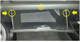
Open the glove box completely and with both hands on each top corner and slide your fingers so force can be applied towards the inside to unhinge the retaining lugs and therefore be able to remove the unit.
