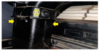
For accesing the cabin filter housing the air duct needs to be removed. With both hands on each side apply force and squeeze to remove the air duct.
