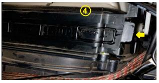
Proceed to unclip on both side to remove the cabin air filter tray.
