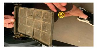
Cabin air filter tray looks as shown in above picture. Clean the area and slide in the new cabin air filter making sure it is facing in the right air flow direction indicated on the filter. Refit all the components in reverse order.
